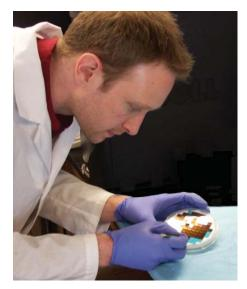
In the Biosensor lab, Ryan Buckmaster exams microfabricated gold and silicon electrode arrays for cell-based biosensor devices.
