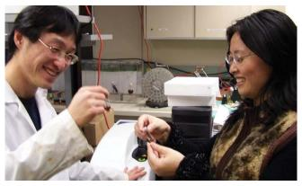
Chen Fang and Miqin Zhang visually inspect the colloidal stability of a synthesized nanoparticle suspension. The equipment shown in the background is a dynamic light scattering instrument which enables measurements of nanoparticle hydrodynamic size and zeta potential.
