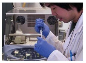
Matthew Leung extracts RNA molecules from stem cells grown on engineered scaffolds in order analyze the cell differentiation using real time PCR
