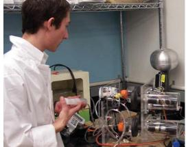
In a Tissue Engineering lab, Michael Rossol tests a bioreactor engineered for dynamic cell culture applications. This instrument enables testing of scaffolds in an environment where the cell chemistry and mechanics more closely resemble In Situ conditions.
