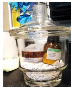
KBr is hydrophilic. The powder and any pellets should be kept in a dry place.
