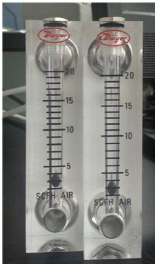
Fig. 2 Chamber and sample purge flow meters
