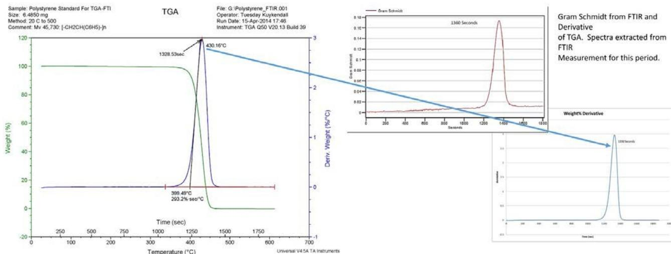
**Fig. 15 Comparison of Gram Schmidt and Wt. % derivative of Polystyrene Decomposition**
