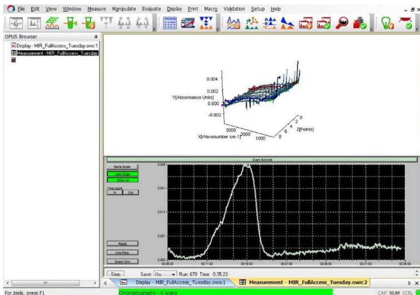
Fig. 14 OPUS 3D scan. Shows scan after 40 minutes. Peak is the Gram Schmidt
