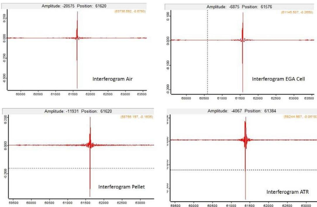
**Fig. 9 Various Interferograms. Note the different amplitudes.**
