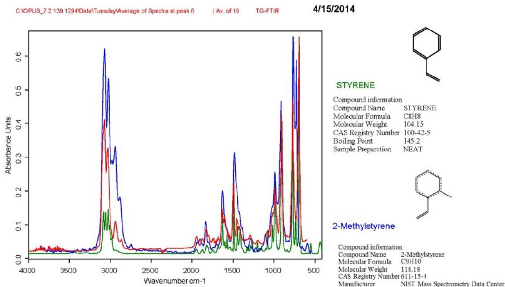
Average of spectra extracted over the period determined by Gram Schmidt and TGA derivative.
