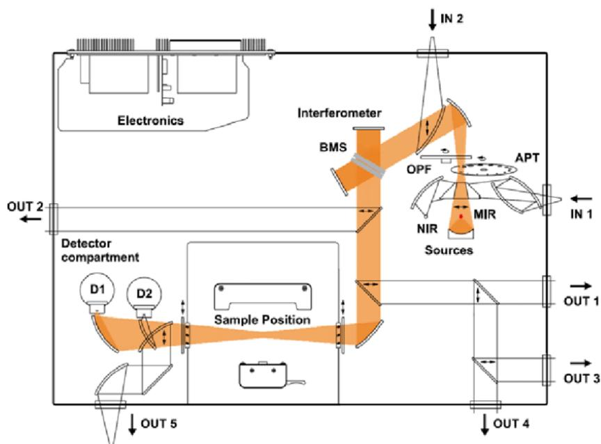
Figure 2 – schematic of the Bruker Vertex 70 (Bruker.com)
