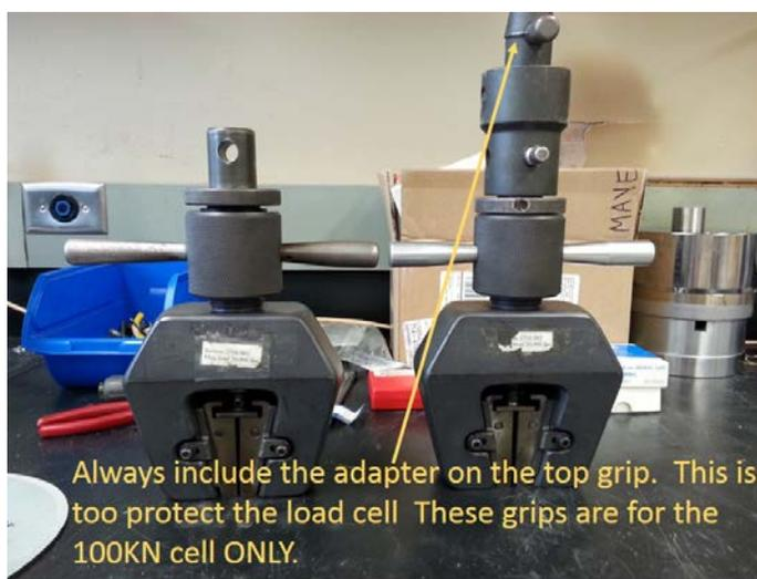
Fig. 3 Tensile grips for 100 KN load cell
